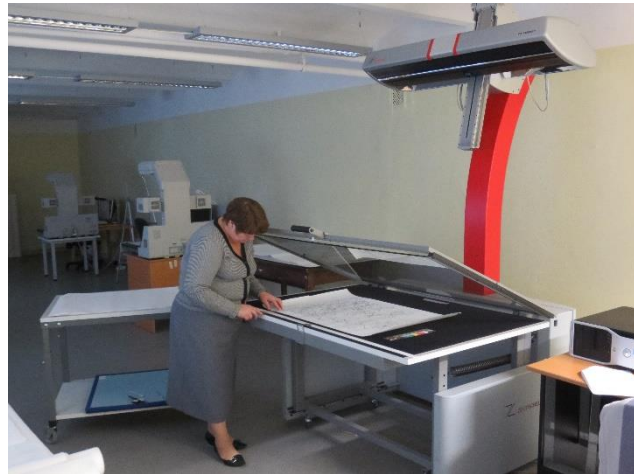
Figure 2. Scanning the Map with Zeutschel Omniscan 14000 Scanner
